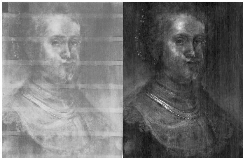
Figure 3. Left: Alan Burrough's shadowgraph taken in the late 1920s, and analyzed by the Rembrandt Research Project. Right: New digital x-radiograph taken at the Conservation Center in 2019, without the interference of the dense cradle
